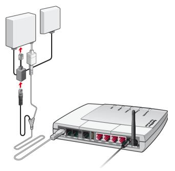
Connecting an analog telephone line to FRITZ!Box Fon WLAN
