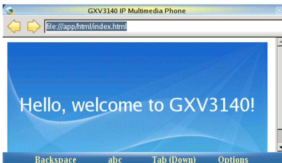
Users can then press F4, corresponding to the “Options”, to move “Forward” and “Backward” on web pages. By selecting “URL” under “Options”, the user can enter the URL of a website. The user can press the F3 button which corresponds to the Tab option to toggle the cursor. Similarly, users can choose “Zoom” under “Options” to zoom in and zoom out of a webpage. Select “Exit” to exit the web browser. The figure below shows the screen of the web browser while visiting a website:
