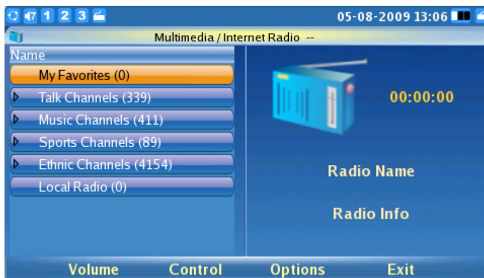
As shown in the figure above, users can then press the F1 button to adjust the volume. From the "Options" button (F3), users can "Open an URL" or "Open URL list" for other Internet Radio stations. The user may also Play/Stop, Mute and Minimize the Internet radio. The user can press F4 to Exit the Internet Radio application.
