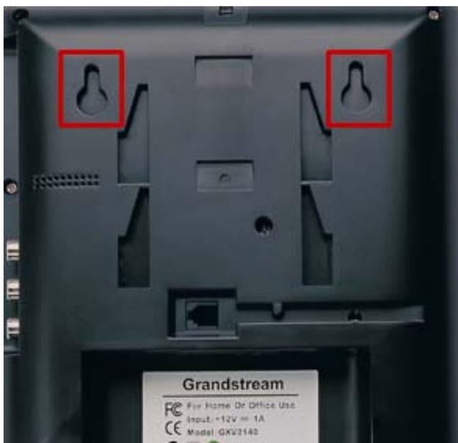
The phone can be mounted on the wall via the two slots on the back of the phone.
