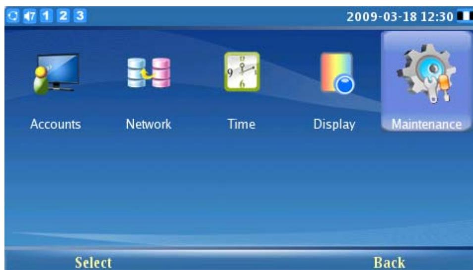
Step 3: Press “Select” (F1 or the OK button) to access the Maintenance page. In the Upgrade tab, press the Down arrow twice to select the Factory Reset option. (Shown in the figure below)
