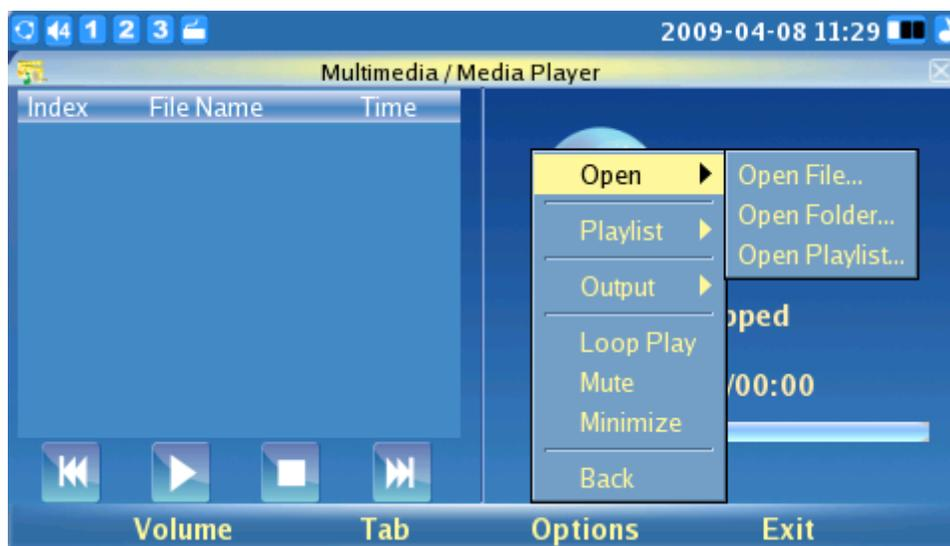
As shown in the figure above, press F1 to adjust the volume of the media player (Navigate by using the Up and Down buttons). Press F2 to enable the “Tab” option, this allows the user to move the cursor between the four buttons: “Previous”, “Play”, “Stop” and “Next”.
