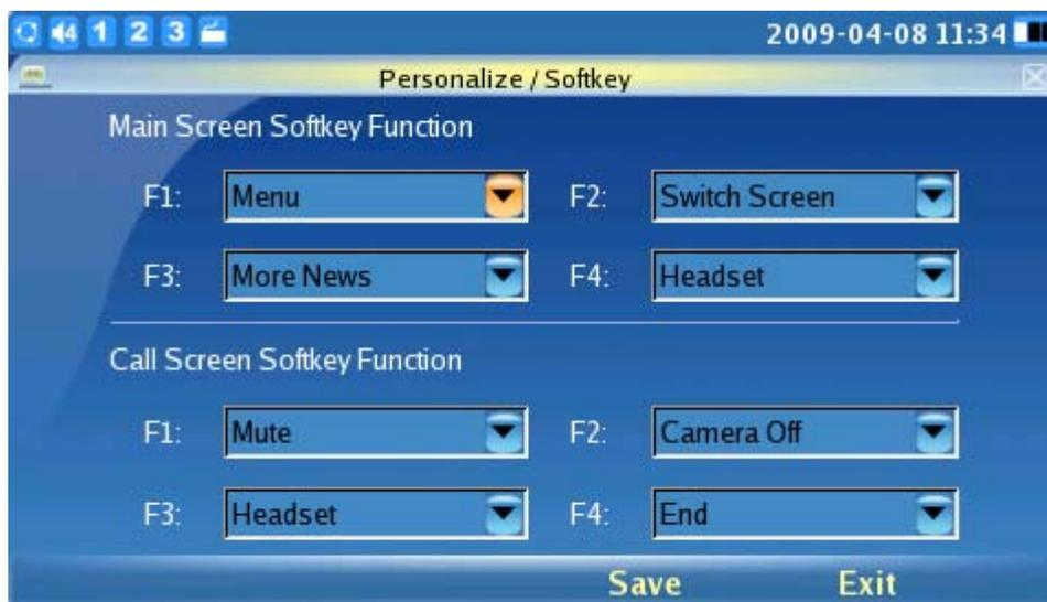
Note: Selecting the “Snapshot” option for one of the softkey functions for the Call Screen lets you capture a snapshot of the remote party during the call. This picture will be saved in the “screenshot” folder and can be used as a picture icon for the contact in the Phone Book.
