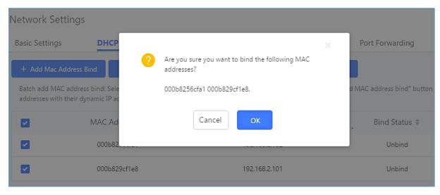
Figure 16: Batch Add MAC Address Bind
