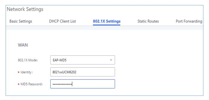
Figure 18: UCM6200 Using 802.1X EAP-MD5
