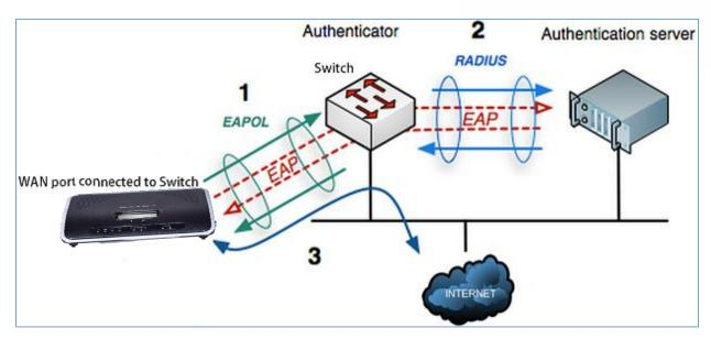
Figure 17: UCM6200 Using 802.1X as Client
