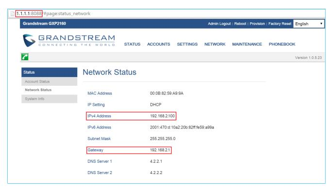
Figure 23: GXP2160 Web Access using UCM6202 Port Forwarding
