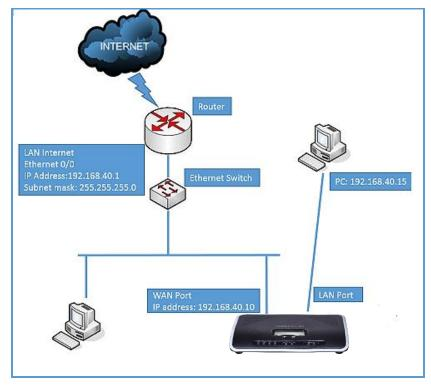
Figure 12: UCM6202 Network Interface Method: Switch
