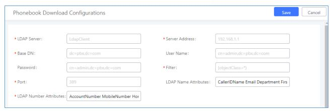
Figure 42: LDAP Client Configurations
