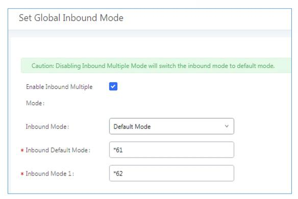
Figure 121: Inbound Route - Multiple Mode Feature Codes
