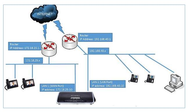
Figure 13: UCM6202 Network Interface Method: Dual
