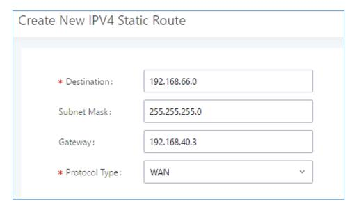
Figure 20: UCM6204 Static Route Configuration
