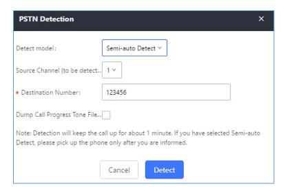
Figure 102: UCM6200 PSTN Detection: Semi-Auto Detect
