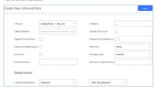
Figure 164: Configure Inbound Rule for Fax
