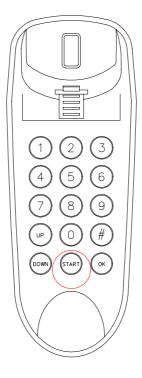
Press the [Start] button at the bottom of the UP-90 USB phone.
