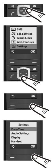
In idle status, press on the right side of the control key to display the main menu.
