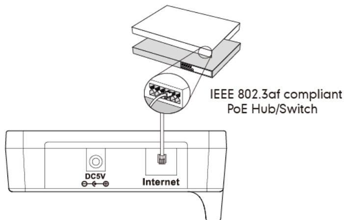
**Note** If in-line power is provided, you don't need to connect the AC adapter. Make sure the switch/hub is PoE compliant.
